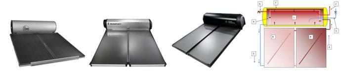
Roof-mounted systems have the collectors on the roof and the solar storage tank is installed above the collectors. No pump is required as heated water moves in a thermal current from the collectors up into the solar hot water storage tank. The water in the collectors is mixed with an anti-freeze/anti-boil liquid. Therefore, the water that moves between the tank and collectors never mixes with the water that you use inside your home.
