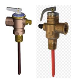
When water is heated it expands and increases the water pressure inside closed vessels like a solar hot water storage tank. The PTRV relieves the excess pressure that builds up inside the solar hot water storage tank when the water is being heated by the sun or booster.
