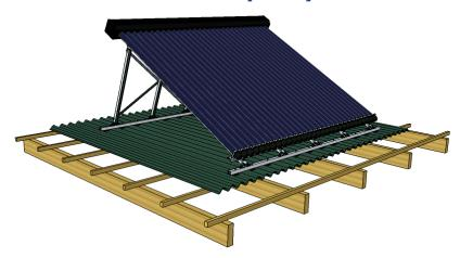
Pitched roof frames are an integral part of solar hot water efficiency and longevity. To gain maximum solar hot water efficiency during periods of high hot water demand (winter), the collectors should be pitched to face the winter sun. At Canberra's latitude the best angle is  $45^{\circ}$  –  $55^{\circ}$  from the horizon.
