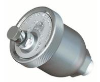
The auto air bleed valve allows air and super heated steam to escape from the collectors. These have a life of around 5 years. They will leak water onto your roof when they fail. These are not always integral to the operation of your solar hot water system.
