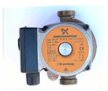
The solar hot water pump moves cool water from the base of the storage tank up into the collectors to be heated, via a flow pipe. The force of the cool water entering the collectors pushes the heated water back to the solar storage tank via a return pipe. The pump does not pressurise the system. It circulates water through the system. The on/off function of the pump is determined by the solar hot water controller.
