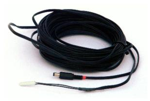
The collectors have a sensor that is wired back to the controller. It tells the controller the temperature of the water in the collectors. Birds will chew the sensor wires that are exposed on the collector. The system will not produce hot water or have frost protection if the roof sensor is broken. Most controllers will have an error code or flashing diode to indicate a roof sensor/collector fault.
